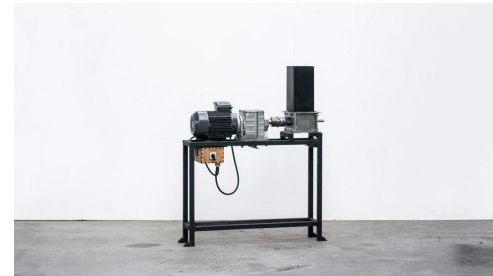
Precious Plastic, shredder
