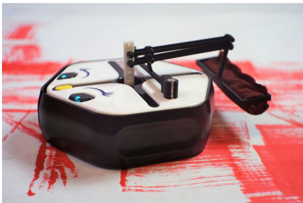
Figure 4. Root with a wide appendage for painting, referred to as the Zamboni
